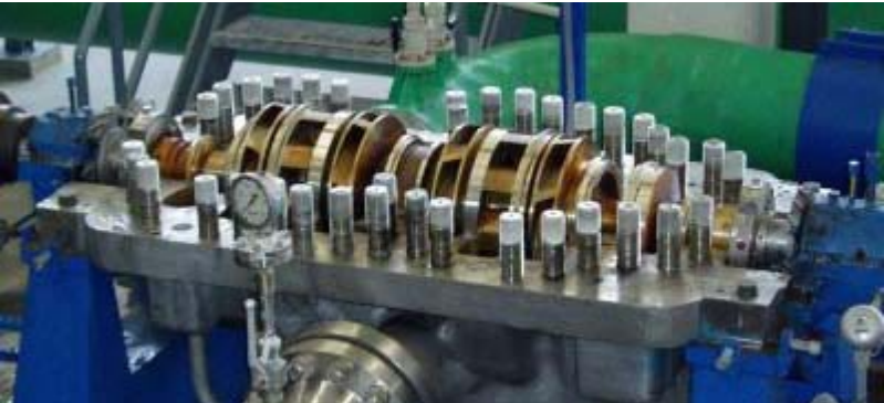
Rotor and interior of turbo pump after opening of casing
