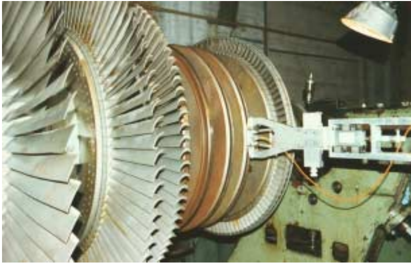
Figure 2 Mechanized ultrasonic examination on the feed pump shaft
