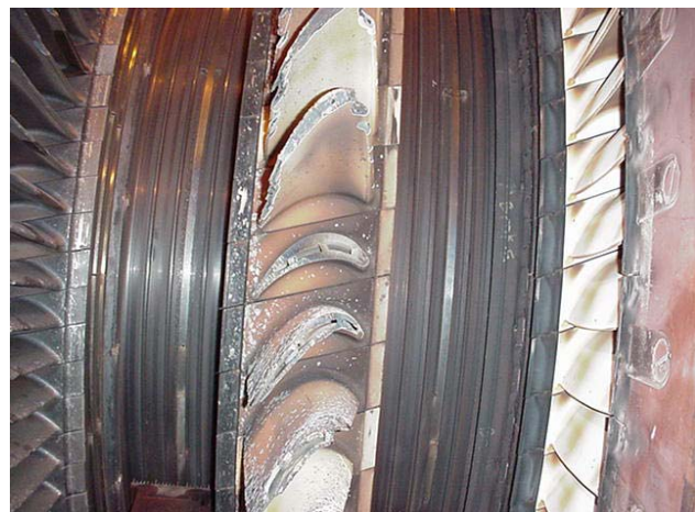
Figure 4 – Advanced Combustion Turbine Compressor and Turbine Blade Damage
