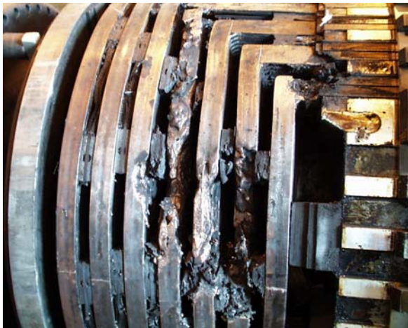
Figure 3 – Melted Generator Windings
