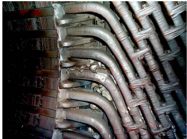
Figure 3 – Melted Generator Windings
