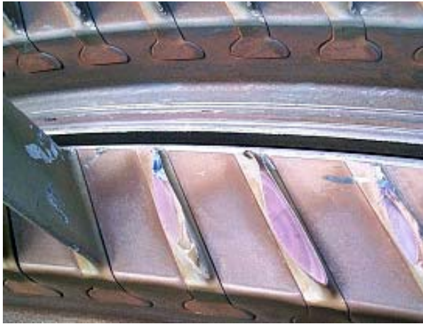
Figure 5 – Advanced Combustion Turbine Compressor and Turbine Vane Damage
