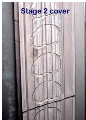
Figure 6 - Advanced Steam Turbine Flowpath Damage/Wear
