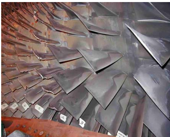
Figure 4 – Advanced Combustion Turbine Compressor and Turbine Blade Damage
