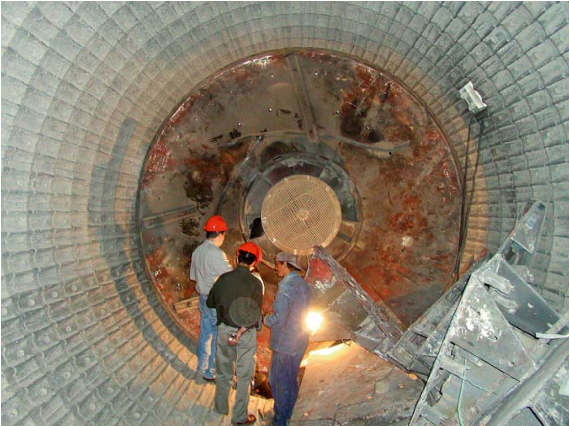
Figure 4: Outlet head viewed from inside the drum
