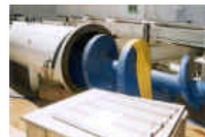
9. Full Face Hard rock Tunnel Boring Machine – NO shield. Hard Rock TBMs are often not fitted with a full shield or pressurised bulk head to protect against subsidence or face collapse where good stable ground conditions are expected.
