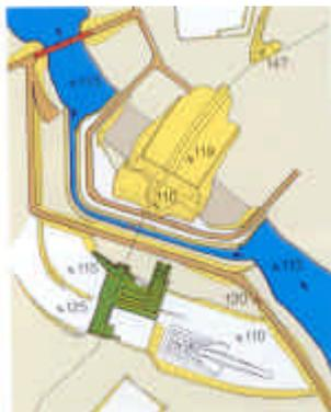
Dam projects invariably involve major river diversion works to provide dry access to the site and river bottom for the foundations. The construction site is usually protected by cofferdams (embankments or cellular cofferdams) and the diverted volumes of water are re-routed in tunnels or open channels in wider valleys.
