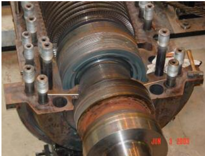
Fatigue Failure Compounded by Condenser Extraction Line Backflow
