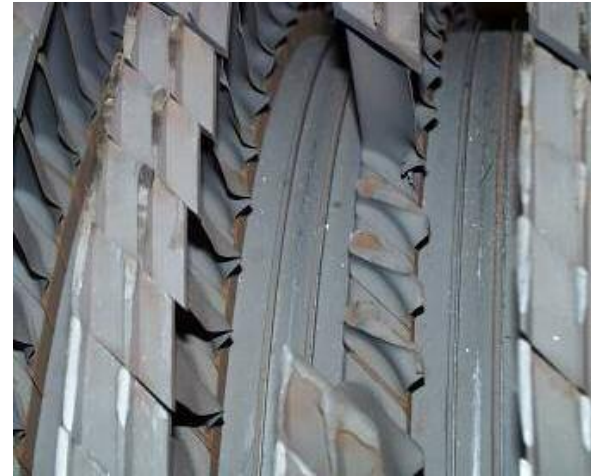
Water Induction Rub Compounded by Attempts to Turn Thermally Locked Rotor
