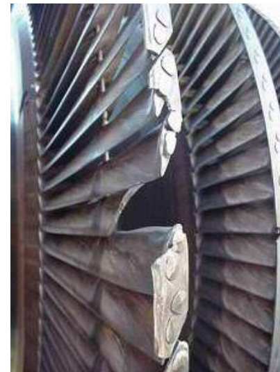
Water Induction Rub Compounded by Attempts to Turn Thermally Locked Rotor
