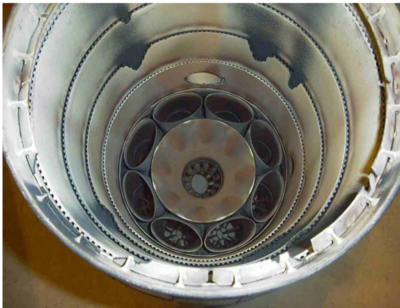
Figure 3 – Combustor Overheating/Flashback Damage
