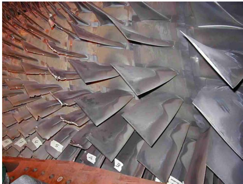
Figure 1 – Failed Compressor Blades
