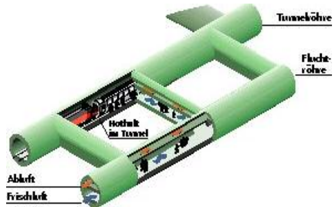
Fig 4: Emergency station in the Gotthard Base Tunnel
