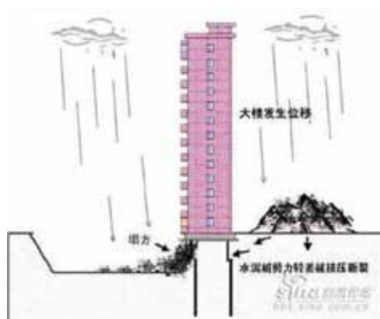
Figure 10. Likely failure mechanism. Shanghai Apartment Building.
