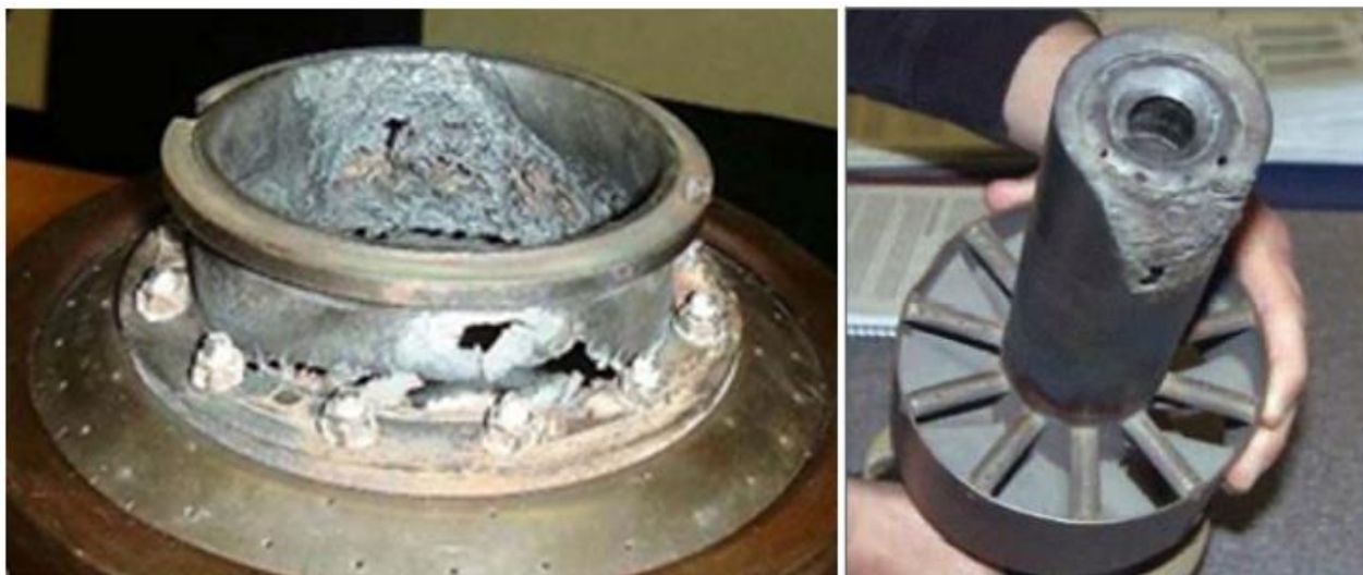
Flashback damage to a fuel nozzle. 96
