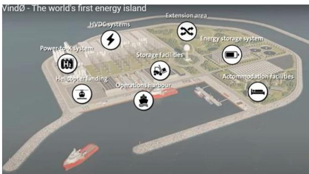
Concept by VindØ includes energy storage, 'power-to-x' facilities such as hydrogen, as well as accommodation, O&M facilities, and HVDC converters for transmission and interconnectors. Source: VindØ
