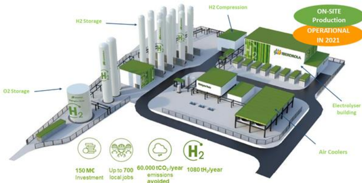
Planned layout of Fertiberia plant. Source: ammoniaenergy.org
