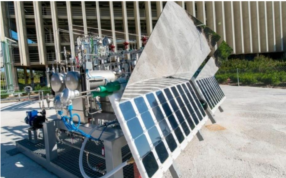
Hydrogen production by photo-electrocatalysis. Source: Repsol
