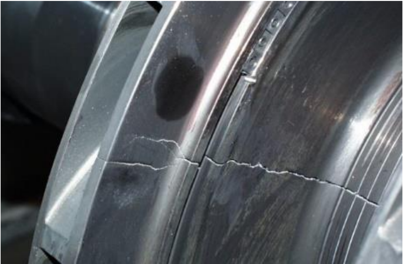
Embrittlement induced crack in rotating machine. Source: Turbomachinery International 145
