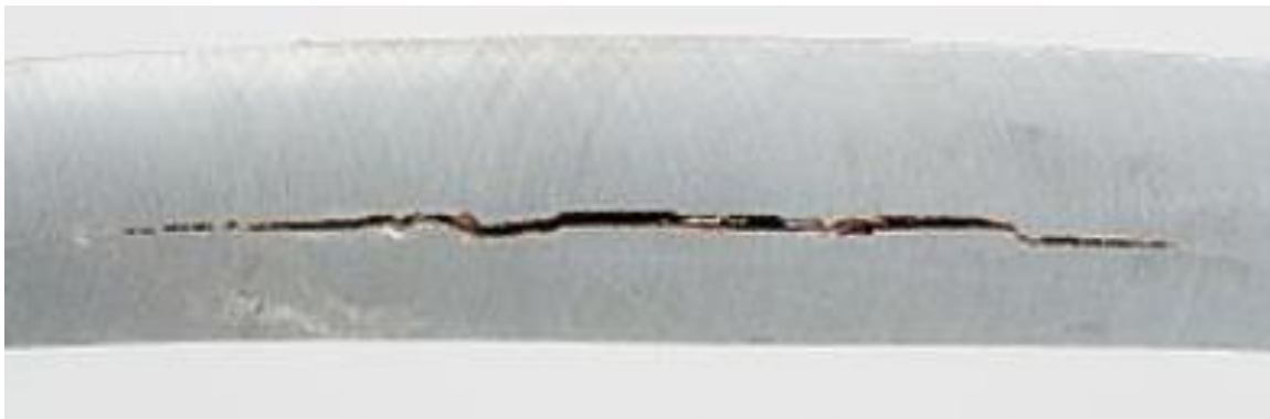
Embrittlement induced crack 144 .
