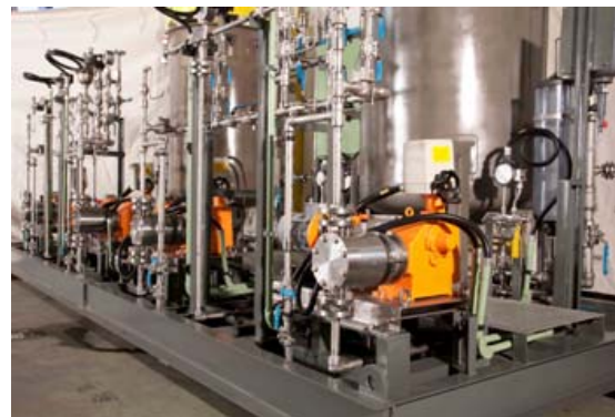
Photograph 7: Skid dosing system. Courtesy ProMinent
