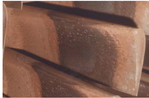
Photograph 4: Rotating blades in a low pressure turbine at first condensation. The areas with oxide deposits are dry, and the blank metal zone is wet during turbine operation.
