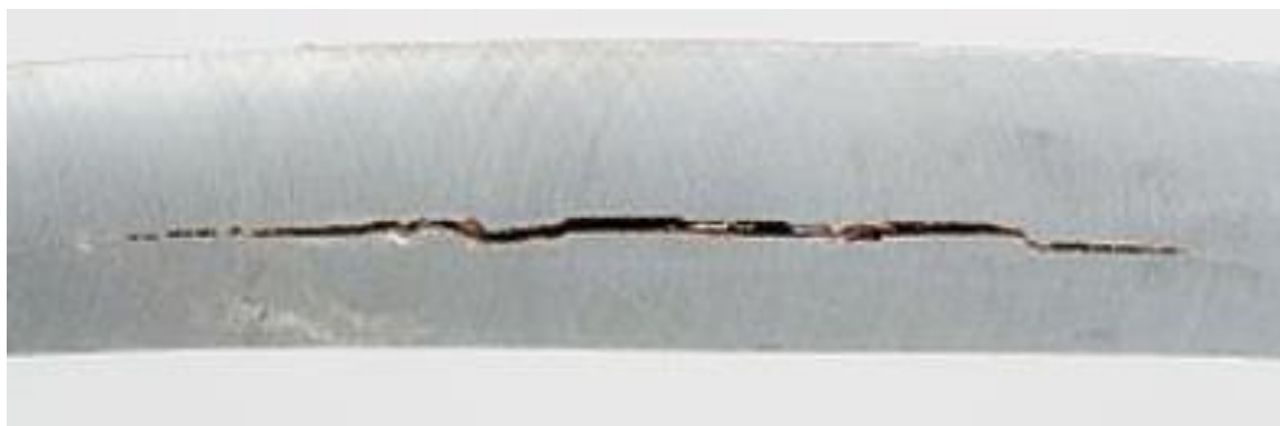
Embrittlement induced crack, Photo by CEphoto, Uwe Aranas 36 .
