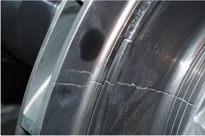
Embrittlement induced crack in rotating machine. Source: Turbomachinery International 40
