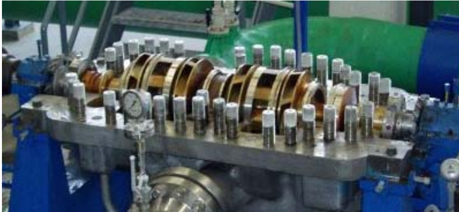
Rotor and interior of turbo pump after opening of casing
