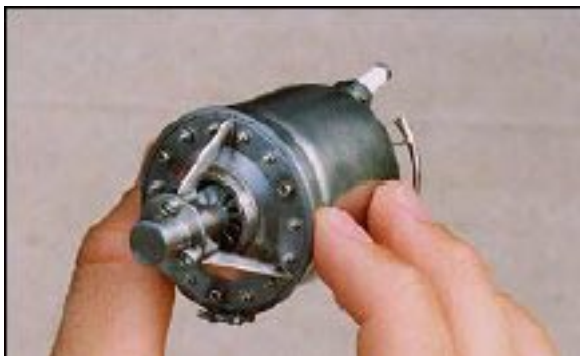
Figure 4: Micro gas turbine developed for US Department of Defence
