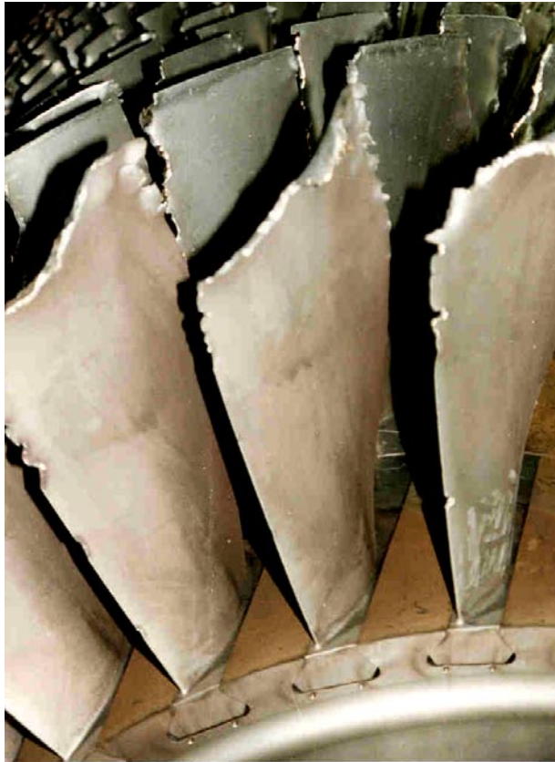
Figure 11: Compressor damage caused by foreign object
