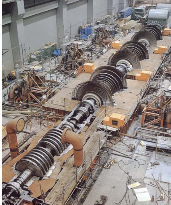
Figure 11 – Multiple Casing Reheat Steam Turbine (Courtesy Hitachi)
