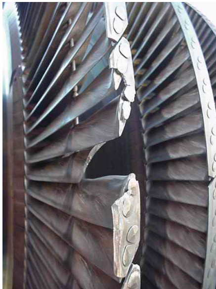
SCC Failure in LP Blade Leading Edge (Flame Hardened Area)
