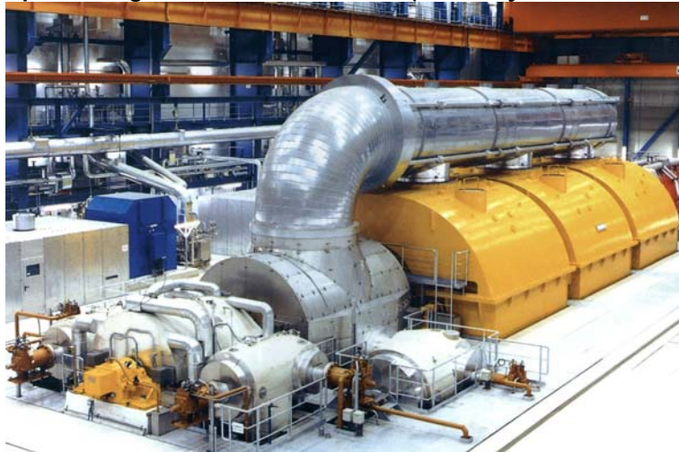
Figure 11 – Multiple Casing Reheat Steam Turbine (Courtesy Hitachi)
