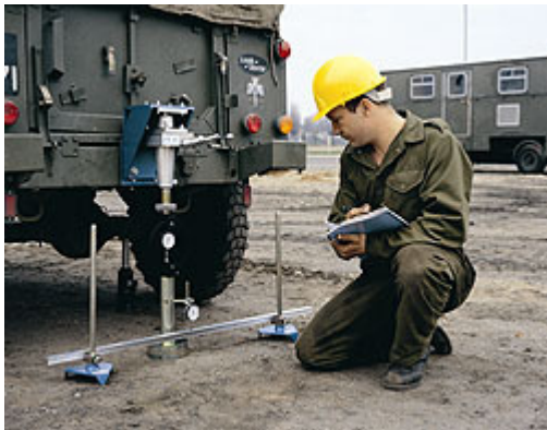
California Bearing Ratio (CBR) test
