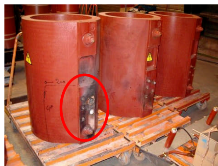
Short circuit in the transformer. Root cause was probably high temperature due to insufficient cooling.
