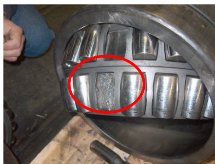
Pitting (wear) on one of six bearings from the planetary stage.
