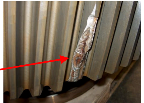
Broken tooth on the low speed gearwheel in a 2 MW gearbox.
