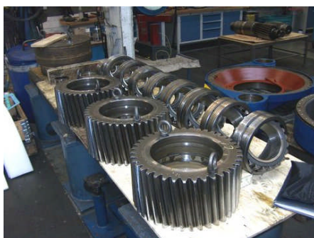
The three wheels and the 6 bearings from the planetary stage of a typical gearbox.
