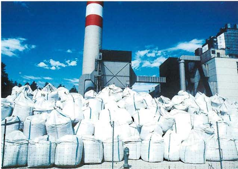
Filtered residues from flue-gas treatment by semi-dry scrubbing present a real disposal problem.
