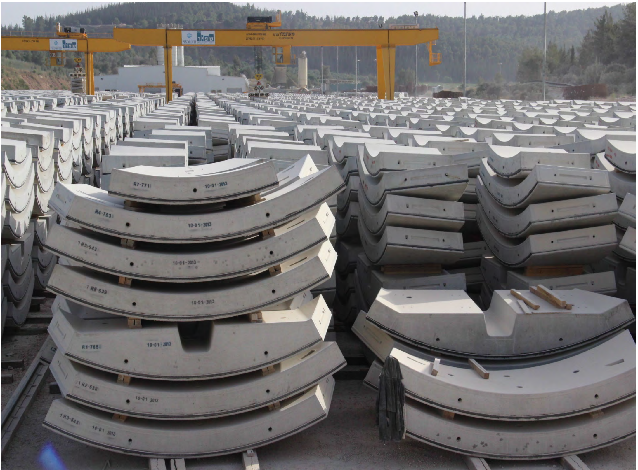
Storage of railway tunnel linings (Alon Eisenberg, Engineers, Surveyors & Loss Adjusters)
