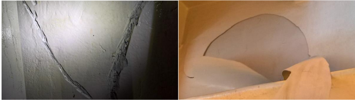
Example of cracked and peeling coating due to varying temperature at the manufacturing site (about 28 °C) and operational site (about -40 °C – 15 °C).
