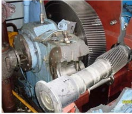
Damaged casing, gears and shafts
