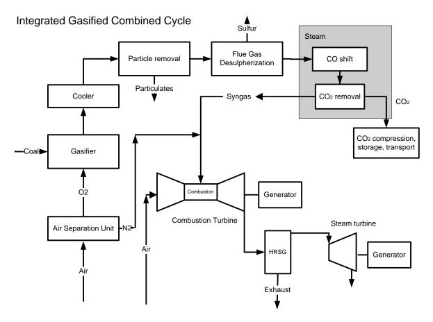
In principle, the individual components of the pre-combustion capture concept have been successfully used in the industry for many years. However, it still remains to be seen if this technology can be applied to power plants with acceptable reliability and availability in parallel with economic operations.<sup>26</sup> With the addition of the new complexity of CO<sub>2</sub> removal there is an even greater amount of uncertainty.
